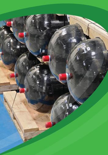
The Largest Diameter Type 3 Cylinders for H≥ Storage
